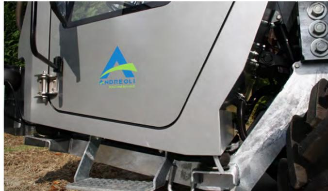
Stainless steel cab with pneumatic suspensions system. Front roll bar for protection against tree branches.
