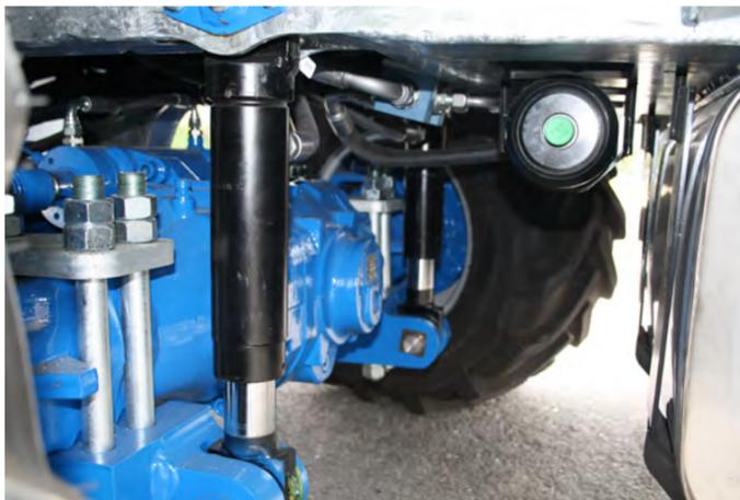
Front + Rear Axles hydraulic suspension system giving the machine a dream like ride. Automatic electronic adjustment of hydraulic suspensions. Automatic leveling of the machine for best stability and comfort.
