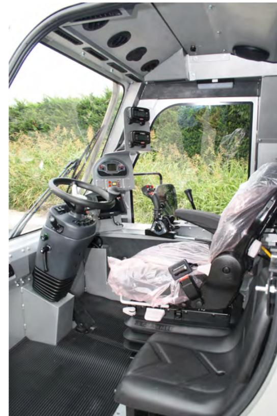
Category 4 cab ensuring maximum protection level for the driver. Chemicals and dust proof cab air filter. Pressurized cab.
